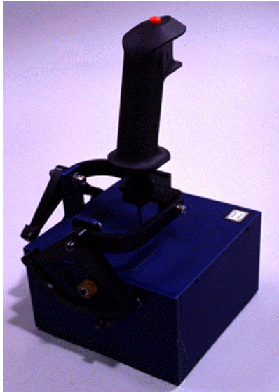
Figure 1.1 Force-Feedback Devices for augmenting on-screen objects. a) Immersion's Impulse Engine b) SensAble's PHANTOM
